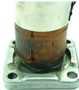
Figure 8: C&D Valve Fuel Hose Flange
