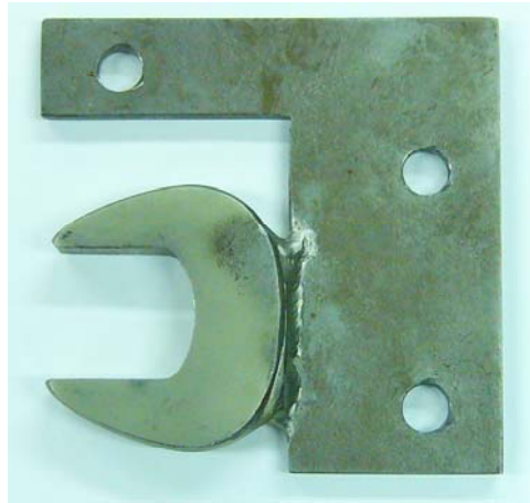
Figure 2: Lower Fuel Manifold Restraining Tool
